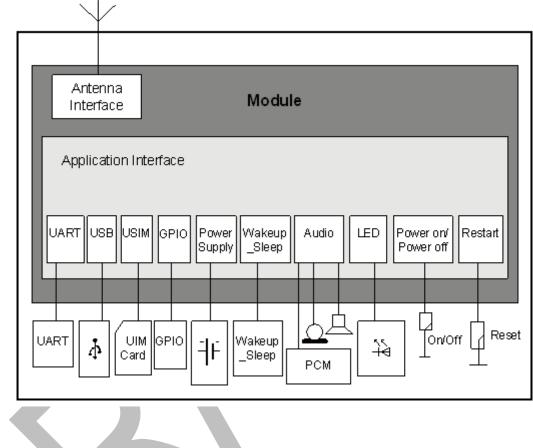
Figure 2-2 Application block diagram of the MC509 module
